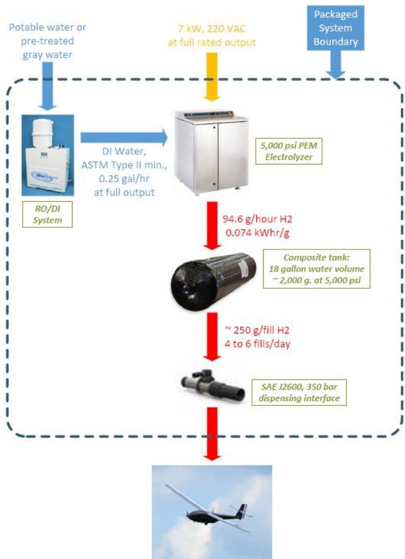
Figure 2: Diagram of system components
