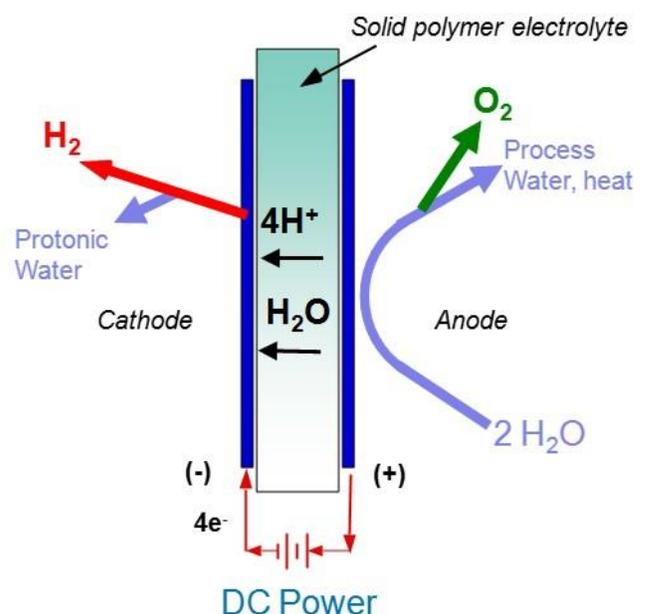
Figure 1: Electrolysis is the splitting of water to produce hydrogen and oxygen gas 3
