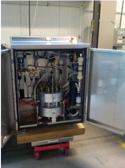
Figure 3: 5,000 psi Electrolyzer System
